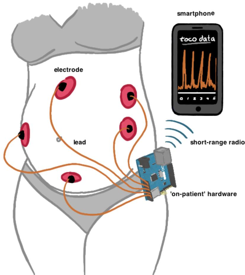
**FIGURE 1.** System-level diagram outlining the hardware setup on the patient as well as the channels by which data will travel from from the patient to the smart-device.
