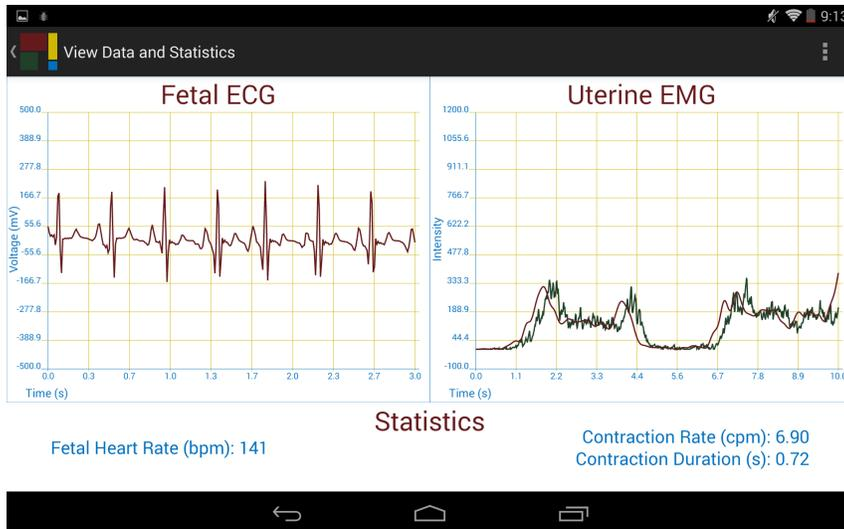
Figure 4 shows the monitoring page of the application. The graph on the left shows a visual representation of the fetal heart signal. The graph on the right shows the uterine muscle signal. Below the plots, the fetal heart rate, contraction frequency, and contraction duration are calculated and displayed.
